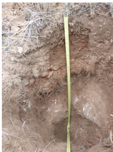
Figure 7. Hand excavated pit for the Stony Upland ecological site, showing the fine-loamy upper profile with a skeletal lower subsurface profile.
