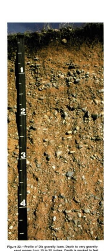
Figure 8. Soil Profile Image-Dix gravelly loam, Cheyenne County, NE. Depth is marked in feet.
