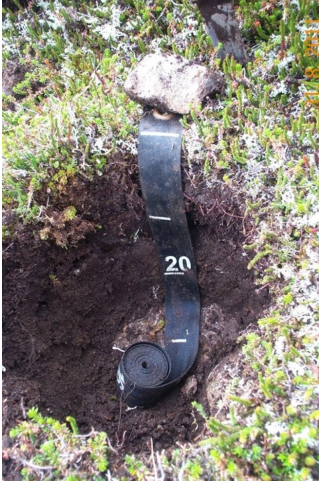
Figure 9. A typical soil profile for this site. The soil is dry, gravelly, and bedrock controlled. This photograph was taken in the Skagway-Klondike Gold Rush National Historic Park, Area.
